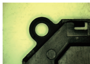
Plastic molded part Under coaxial top light at 0.35x optical magnification
